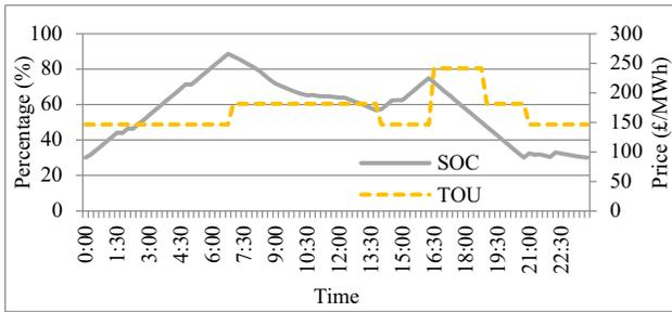
Fig. 8. SOC of battery in normal house.
