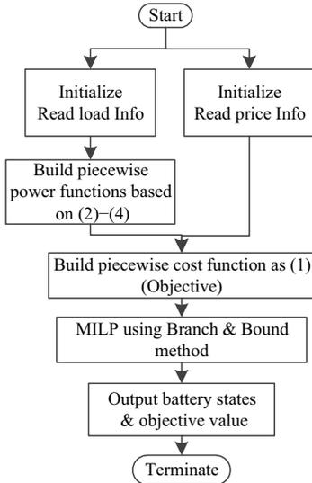
Fig. 5. Flowchart of optimization method.
