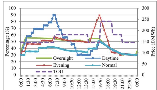
Fig. 14. SOC of larger battery.
