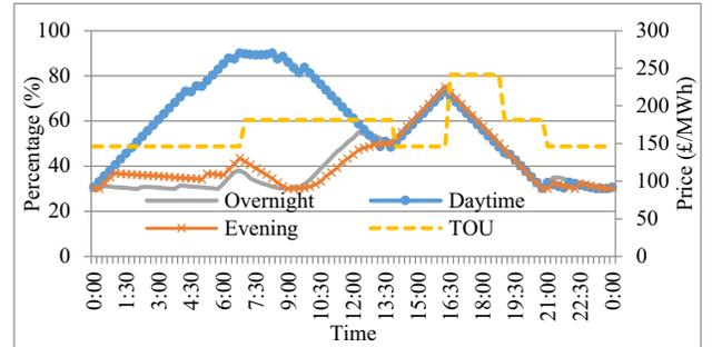
Fig. 17. SOC of electric heating house with large PV output.
