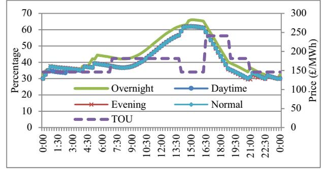
Fig. 15. SOC of battery in EMS system with 89% efficiencies.
