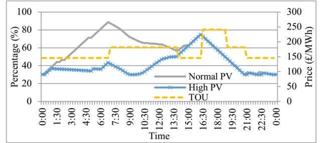
Fig. 16. SOC of normal house with large PV output.
