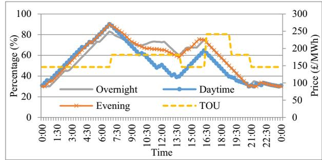
Fig. 10. SOCs of battery in houses with heat load.
