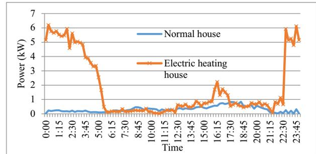
Fig. 1. Demand of houses with and without electric heating
